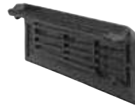
RIGHT HAND INDEPENDENT CLOAKED VERGE TILE (2,7 per m, gauge 370mm) Ref.200.41
